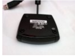
Peel off front two rubber feet
