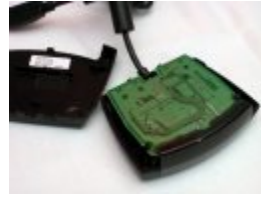
Pry open moulding then unscrew one remaining screw
