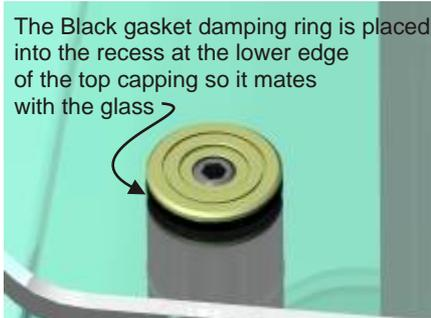
Ensure the M8 x 25mm Stainless Steel allthread is flush with the recess in the top brass capping to allow the black cover cap to be affixed - it must be flush with the top of the capping. Tip: It is recommended to tighten the top cappings by holding the brass top capping and turning the allthread using the allen key together.
